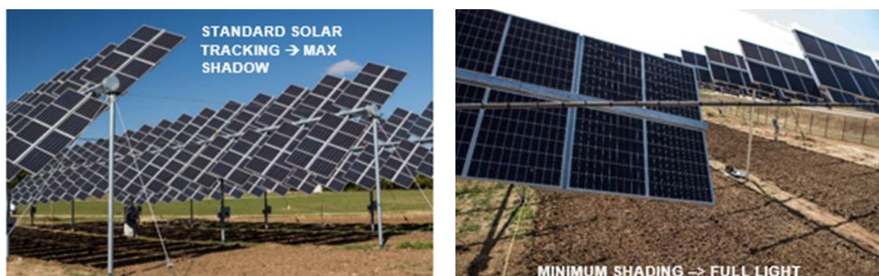
Figure 5: Management of the shadow below Agrovoltaico® tracker 3D
